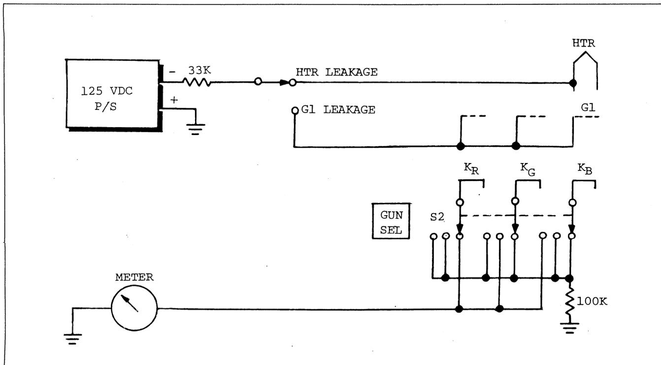
Fig. 3. Model 480 leakage test circuit (simplified).
