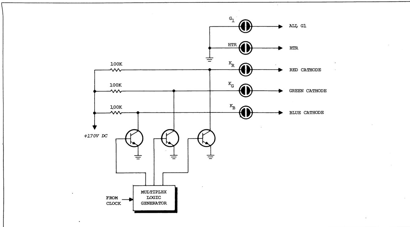
Fig. 9. Model 490 leakage test circuit (simplified).
