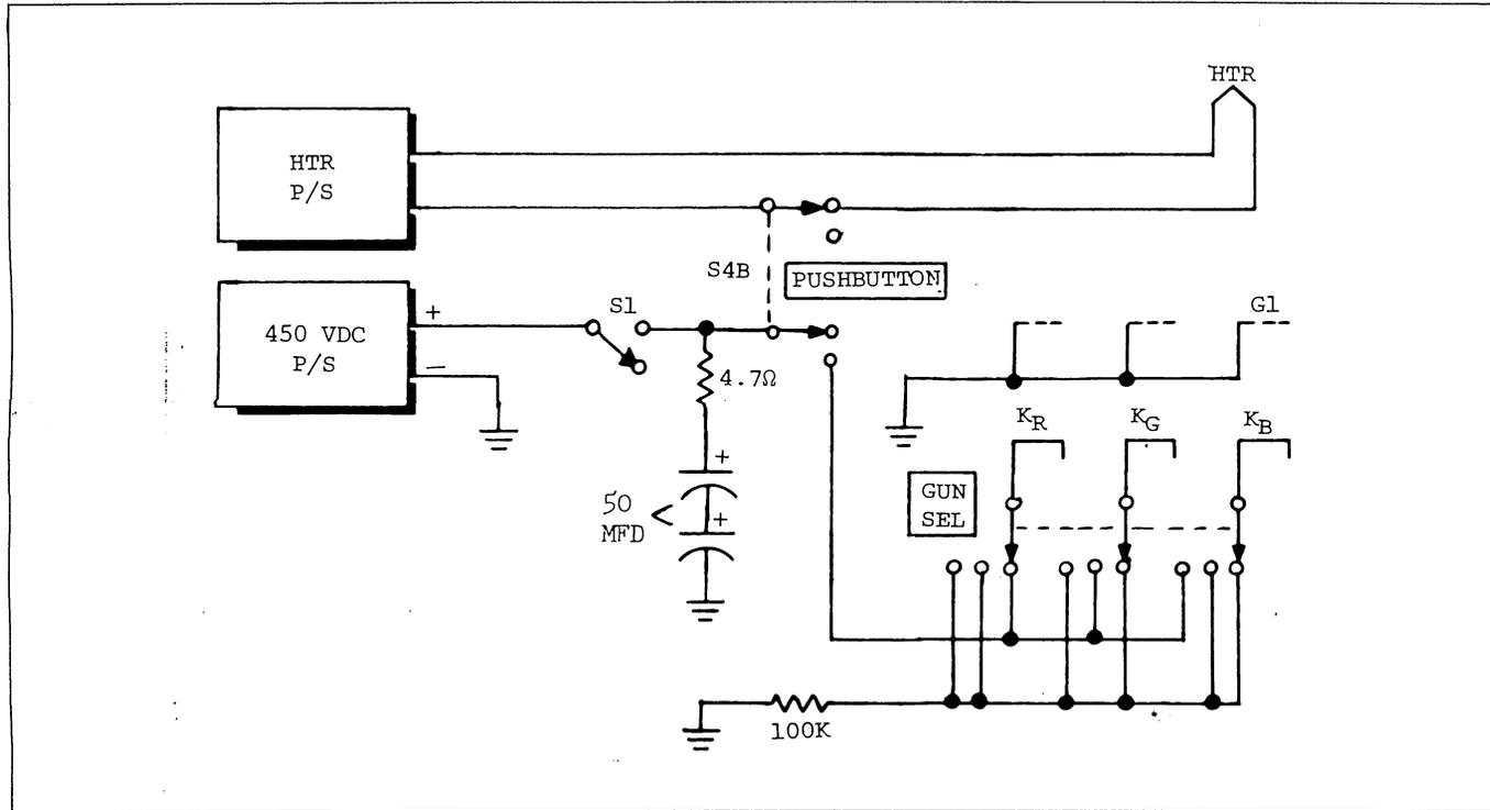
Fig. 5. Model 480 shorts removal circuit (simplified).
