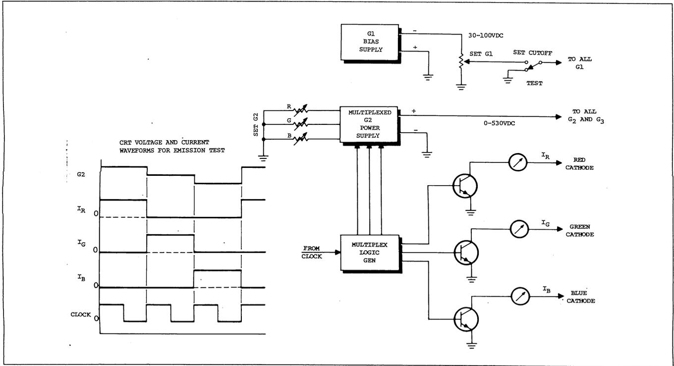
Fig. 7. Model 490 emission test circuit (simplified).
