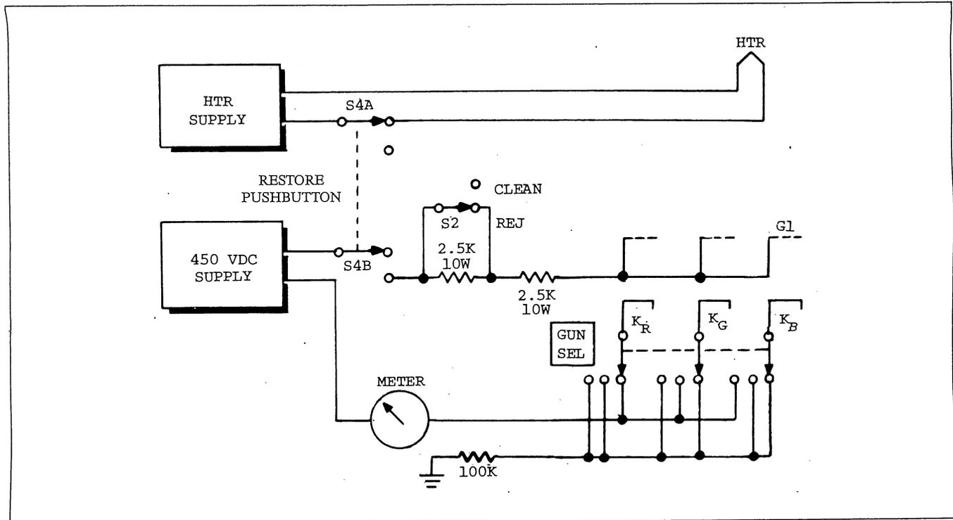
Fig. 6. Model 480 clean, balance, and rejuvenate circuit (simplified).
