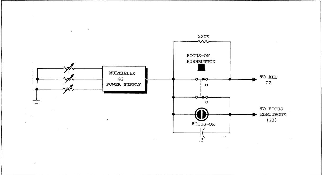
Fig. 10. Model 490 focus continuity test circuit (simplified).
