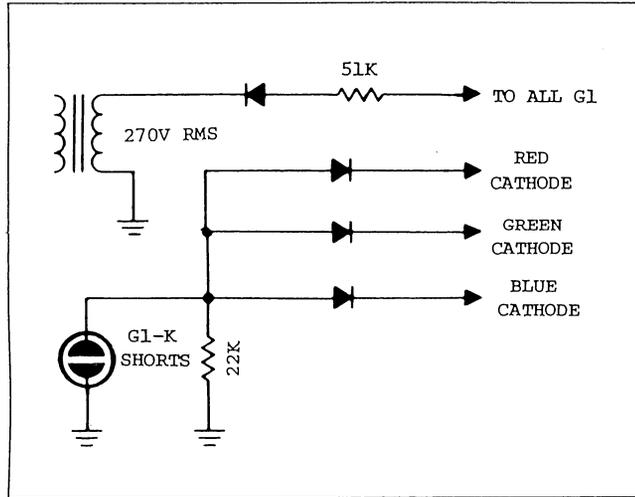
Fig. 11. Model 490 G1-K short indication circuit (simplified).
