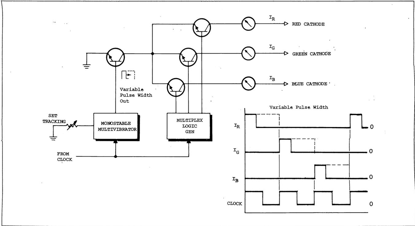
Fig. 8. Model 490 tracking test circuit (simplified).
