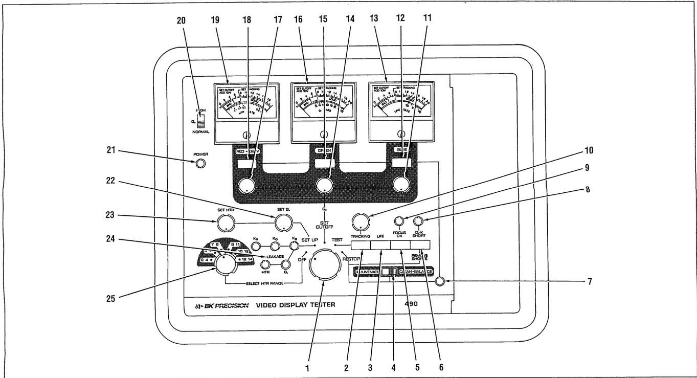
Fig. 2. Model 490 controls and indicators.
