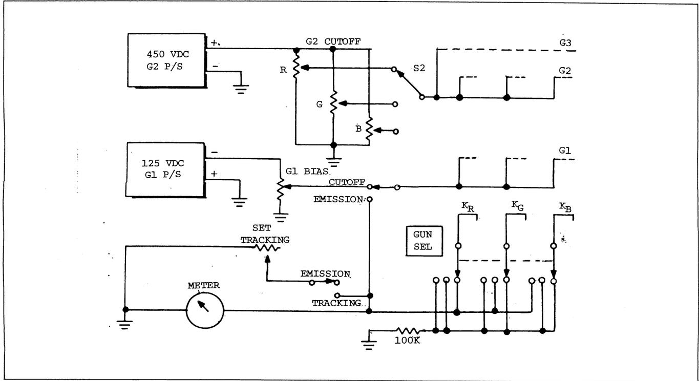
Fig. 4. Model 480 cut-off, emission, and tracking test circuit (simplified).
