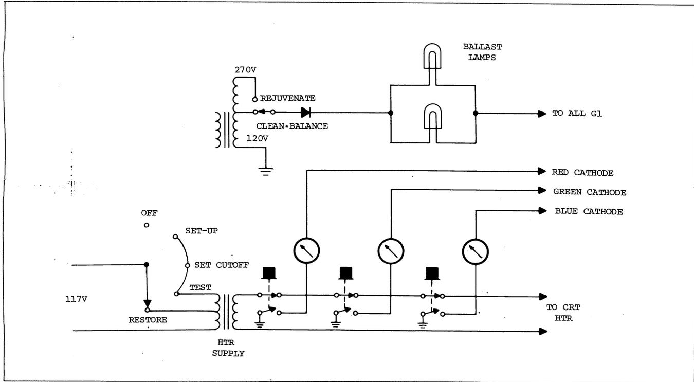
Fig. 13. Model 490 clean, balance and rejuvenate circuit (simplified).
