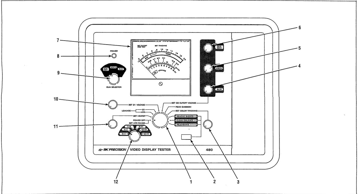
Fig. 1. Model 480 controls and indicators.
