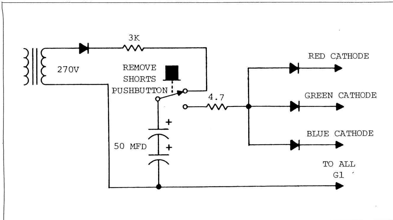
Fig. 12. Model 490 G1-K short removal circuit (simplified).
