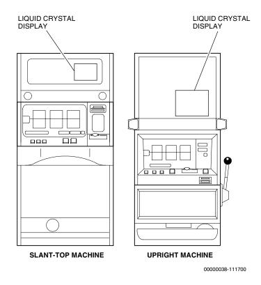
Figure 1-3. Liquid Crystal Display Location.
