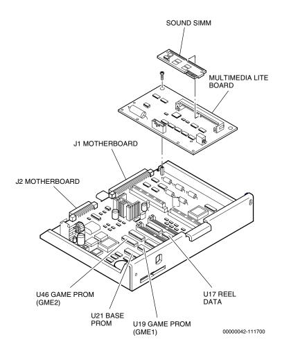
Figure 4-1. Component Locations, Vision Processor Board for Stereo Sound (p/n 755-105-0X)
