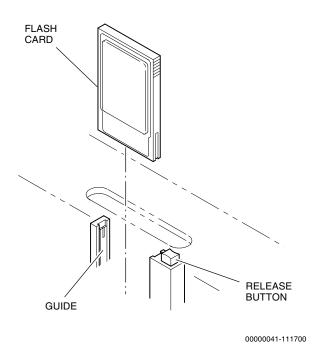
Figure 4-5. Flash Card Installation
