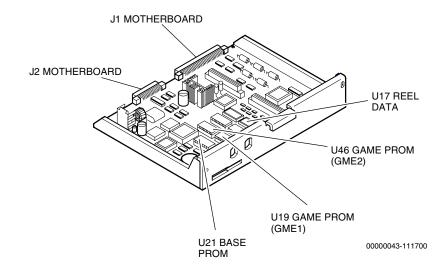
Figure 4-2. Component Locations, Vision Processor Board for Mono Sound (p/n 755-105-0X)
