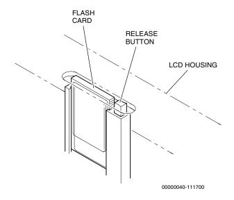
Figure 4-4. Flash Card Removal
