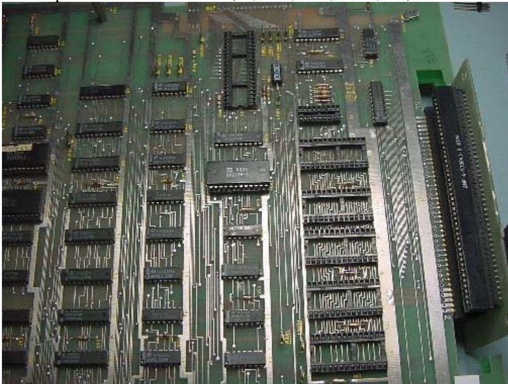
Install kit main board into processor socket 2C & Eprom socket 1F being careful to align the pins properly.
