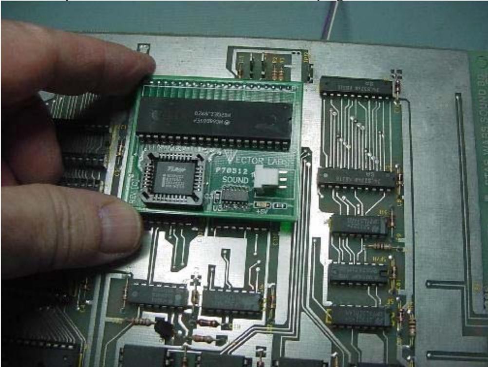
Install the 3 pin cable violet,gre,y,white into the white male connector as shown below.
