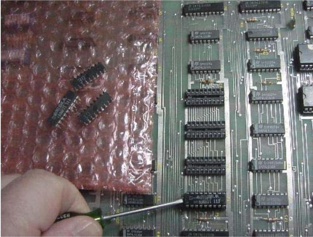
Be careful aligning the pins when installing the Instruction PROM board as shown below.
