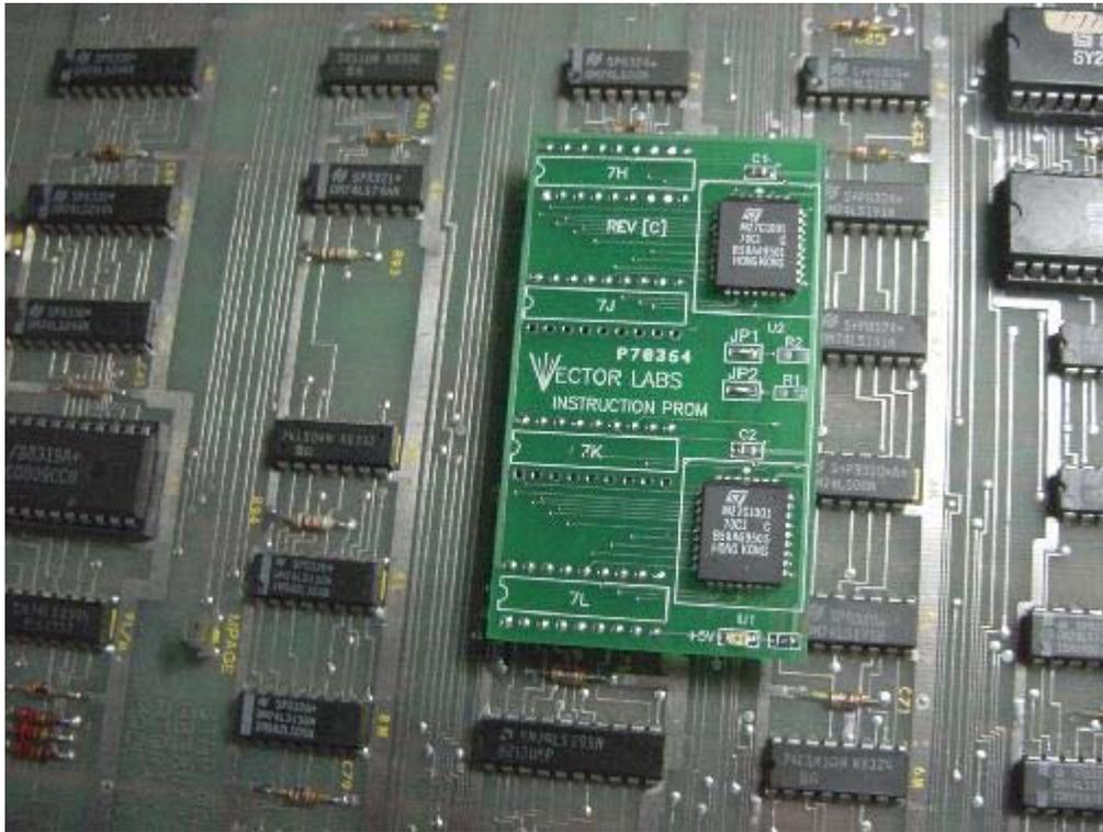
Remove 68B09E processor (2C), NVRAM X2212 (1E) and Eproms from all 5 locations (1F, 1H/J, 1J/K, 1K/L, 1M) as shown below.
