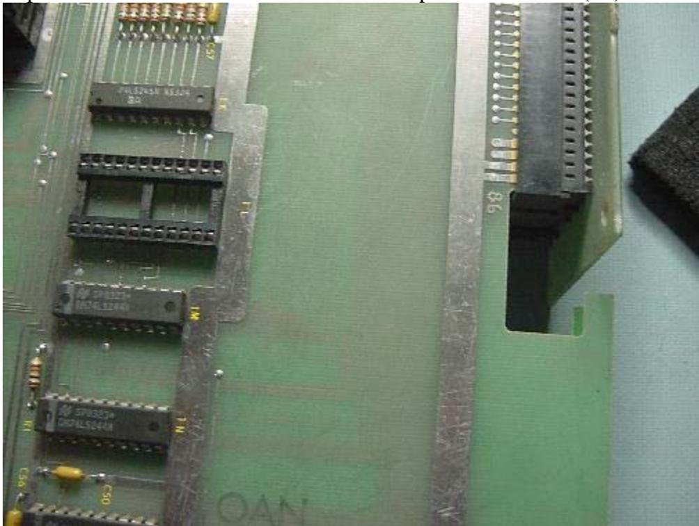
Install the Vector prom replacement board into socket (1L) as shown below.
