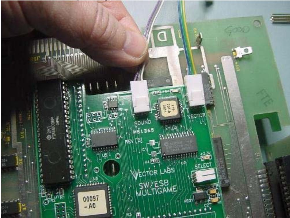
Flip the boardset over and remove the vector Eeprom from socket (1L).
