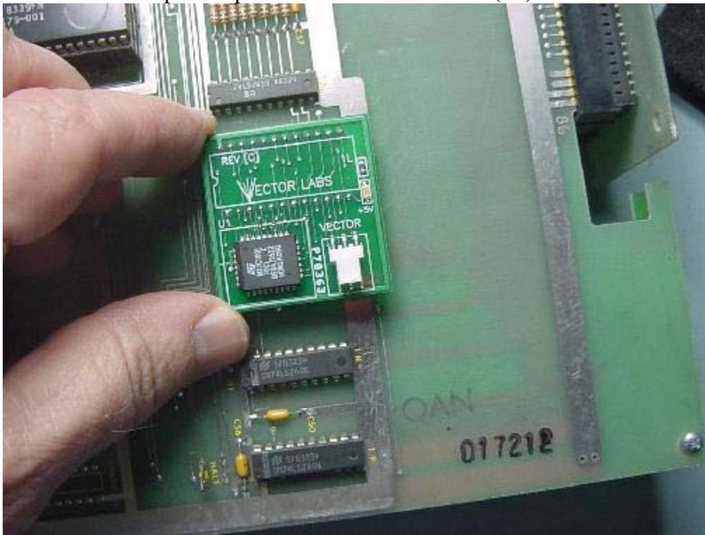
Install the 3 pin cable yellow,green,blue into the white male connector as shown.
