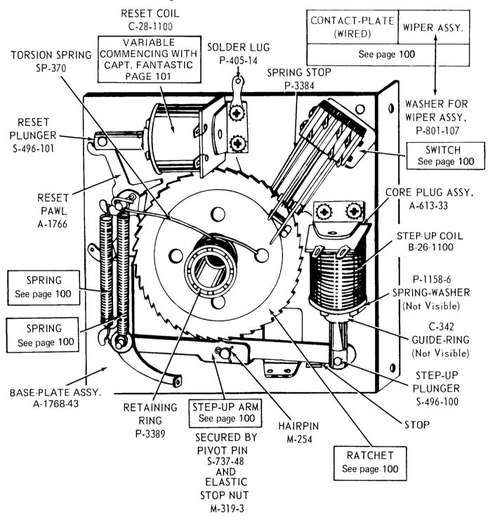
Operate Reset Plunger by hand until Ratchet resets to zero position, i.e., until resetting movement stops. Then operate Step-up Plunger, and while holding Step-up Plunger in, check to see that Reset Pawl rests at base of ratchet-tooth (point at which straight and angular edges of tooth meet). If Reset Pawl is not at base of tooth, adjust Spring-Stop (P-3384) until Ratchet moves into position to permit Pawl properly to engage tooth, as described. Then check unit
