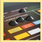
Obviously a key element to the game! These are sealed switches that aren't made any more. The start buttons are illuminated in red; the fire buttons are standard. You can also find these buttons on the old Atari *Sprint* and *Asteroids* cabinets. Getting hold of replacements is really difficult, and as they are sealed units, they cannot be fixed. When they go, they go!
