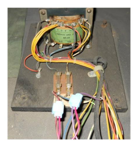
Pictured is a Space Invaders upright transformer where we tapped into 120v. Note: The wires you tap into can vary from game to game. In cocktail cabinets, we simply tapped into the 120v wires going to the cooling fan.
