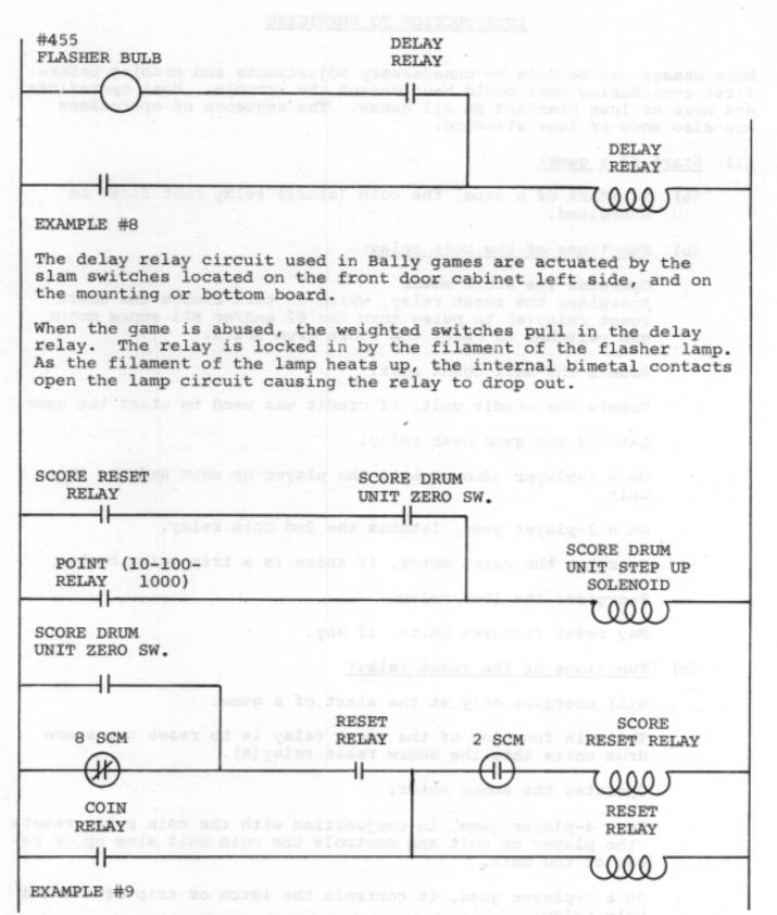
When the coin relay switch is closed, the reset relay is pulled in starting the score motor. The reset relay will stay locked in until all the score drum units advance to zero, and when #8 score motor cam switch is actuated. As long as the reset relay is energized, the score reset relay will pulse thru #2 score motor cam. During the game reset time the score drum units will advance until the score drum units zero switch opens.
