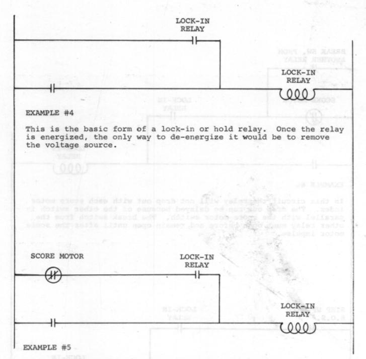
This lock in circuit will drop out when ever the score motor turns. The score motor switch is usually a #8 or #10 cam switch.
