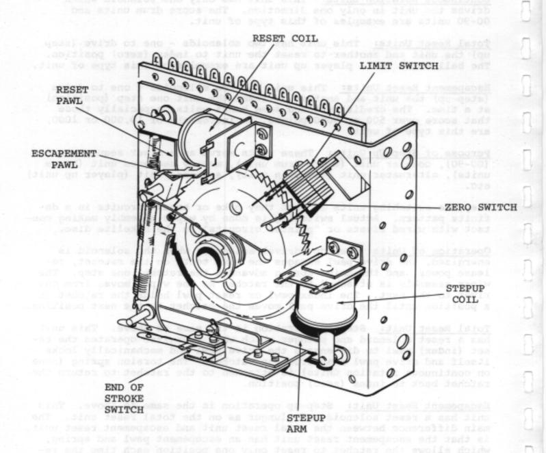
Other Bemes: Stepper Unit, Rotary Switching Unit, Step Switcher ..
