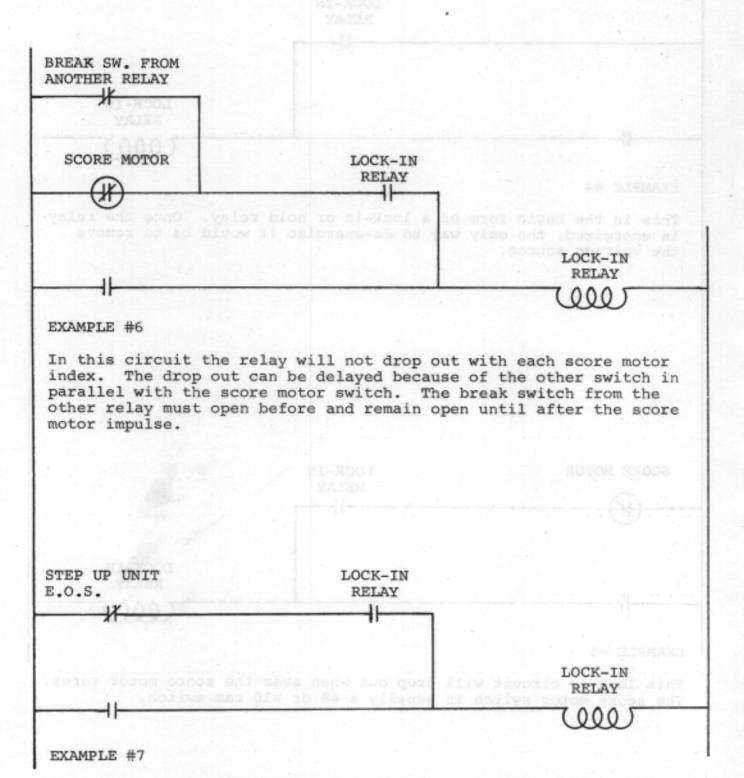
The relay is locked in through a step up unit end of stroke switch. The step up unit must advance for the relay to drop out. A typical example of this circuit is in the point relay (10,100,1000) lock in circuits.
