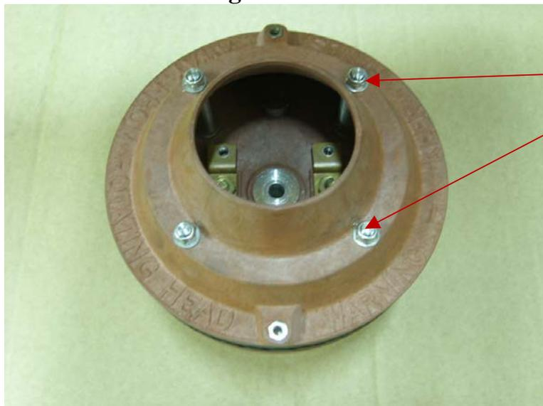
Remove 4 nuts and washers and remove the spin head top cap.
