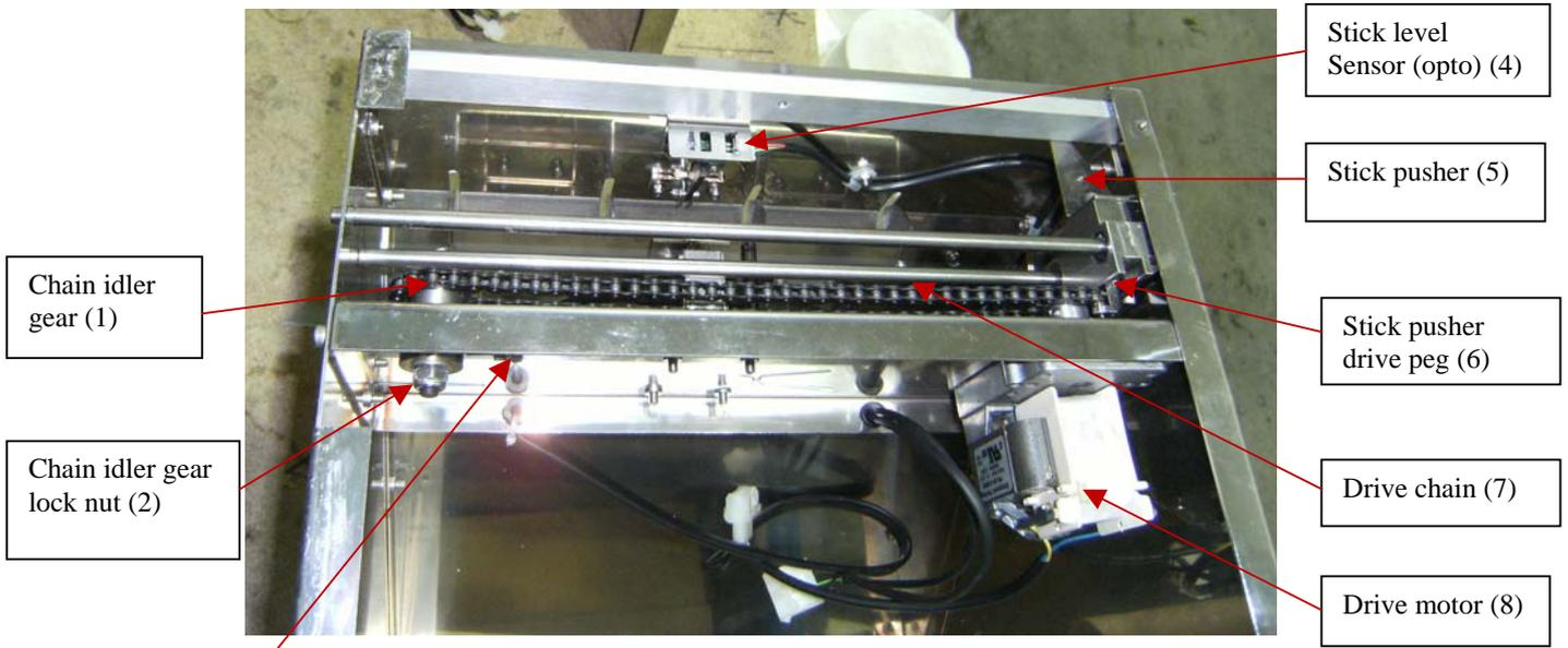
**Fig16b Detail of stick pusher mechanism.**
