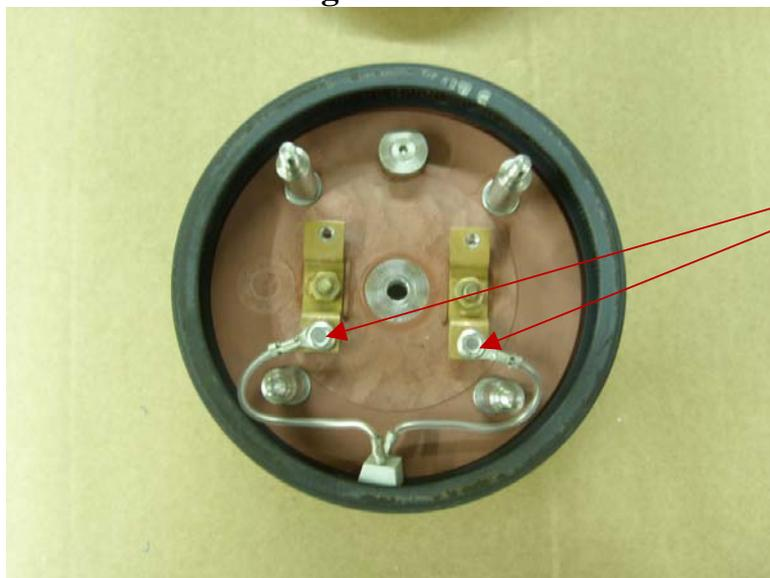
Remove element screws and remove floss band and element as one unit.
