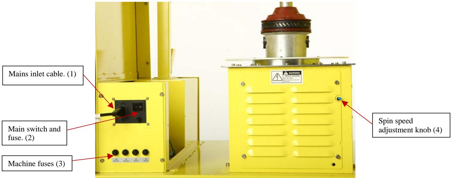
**Fig 3b. Transformer enclosure.**
