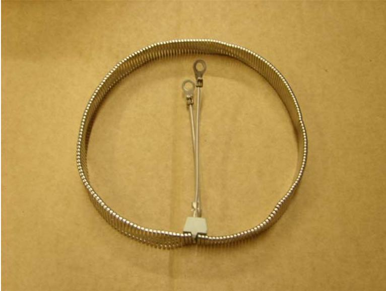
**Fig 19d (Element fitted to floss band)**
